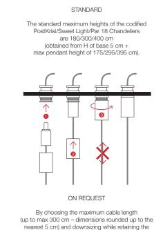
(up to max 300 cm – dimensions rounded up to the nearest 5 cm) and downsizing while retaining the proportions of the standard codes, a custom made composition can be produced. Any further customisation entails a bespoke design requiring a quotation (customized production).
