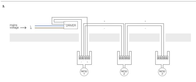
the cable between the lamps is not supplied,
