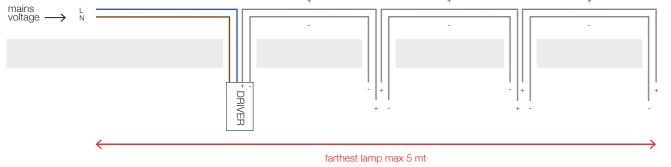
INSTRUCTIONS FOR THE CONNECTION OF MULTIPLE LAMPS RECESSED FOR PLASTERBOARD
